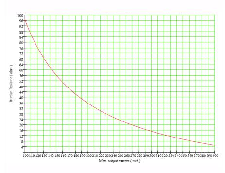
To maintain safe start-up  $\mathbf{R}_{\scriptscriptstyle{\mathrm{M}}}$  must not exceed 30  $\Omega$  during fault condition.
